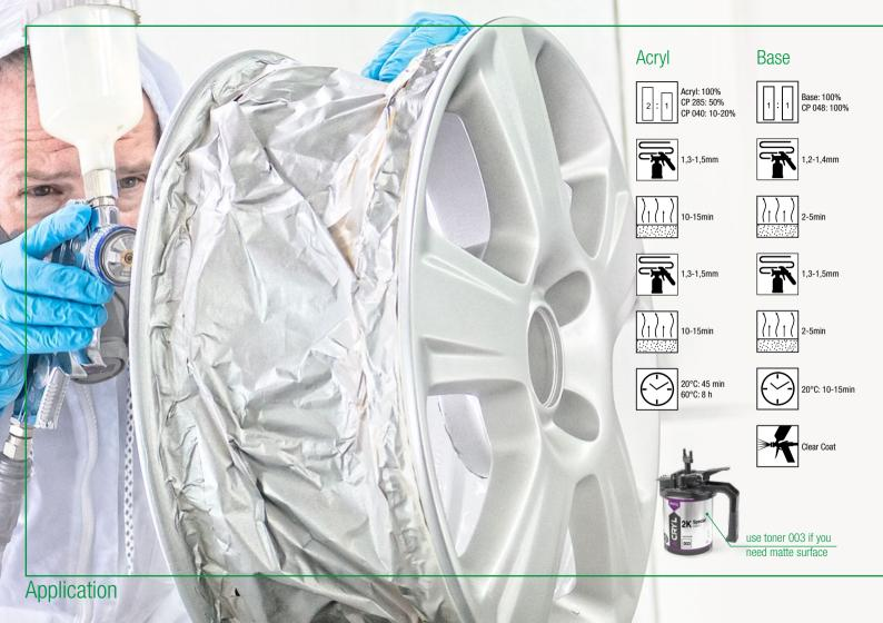
For **Acryl** 2-3 full layers. Time of drying between layers 5-10 minutes. Nozzle size: 1,3-1,5 mm.
